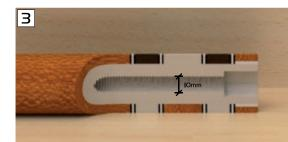
To maintain the possibility of changing weights, remove the bumper and check the diameter of the weight bolt. It must not exceed IOmm to pass into the 3Lobite hole.
